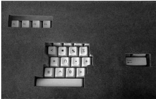
Figure 5. Close-up of the keyboard used in Experiment 2, with the 12 letters on the letter keys replaced by symbols.
