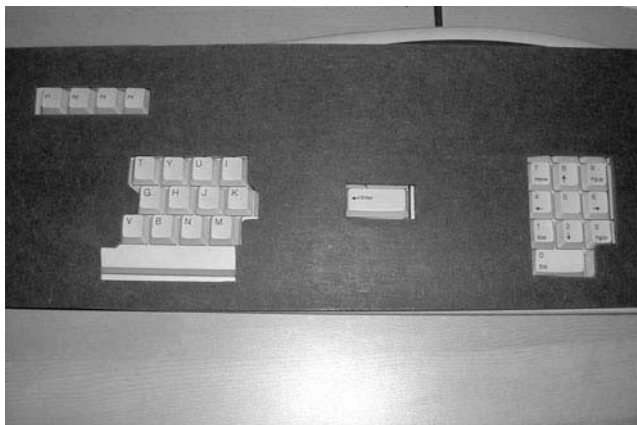
Figure 1. Picture of the keyboard used in Experiment 1, showing the subset of 12 letter keys in use during the experiment.
